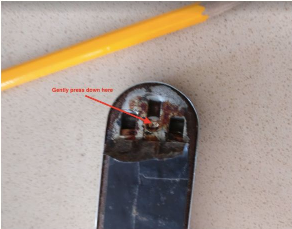
FHC pickup: This mounting tab is accessible externally from the back. You may need to peel back some protective tape to access it. Gently press it down with a blunt point object. I used a blunt pencil.
