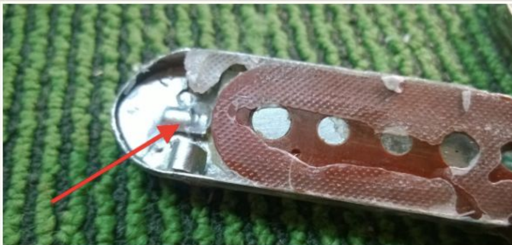
Rhythm Chief: Bending this tab upward will increase rod friction on worn-out mounting holes. You can do this without opening the pickup with a small flathead screwdriver (such as the kind for repairing eyeglasses)
